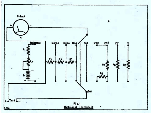
the full scale deflection current and coil resistance of the meter are known.
